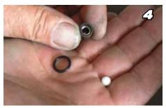
Thoroughly clean the ball, spring and O-ring with alcohol and water. Then clean the seat.
