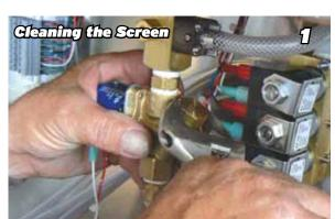
Using your Adjustable Wrench, turn the nut counter clockwise until
