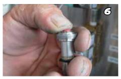
Be sure that the plunger moves in & out freely by pushing with your finger. Replace if needed.
