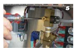
Once you have the injector back together, turn the power back on and turn on your Dog Wash. With selector switch on Disinfectant or Veterinary Shampoo, squeeze shower head handle to see if soap is being pulled. If no soap is being drawn, slowly turn the screw on injector to the right until soap draws. If soap is still not being drawn up, slowly back down the screw and keep going left until soap begins to draw. Turn clockwise to increase pressure, counter clockwise to decrease pressure.
