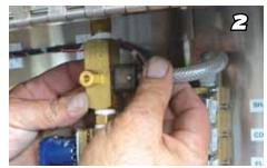
Once screws are removed, carfeully pull out the housing.
