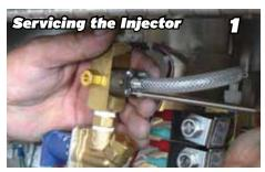
If your Injector gets any dirt in it at all, it will not work. Start by removing the four screws on each corner.
